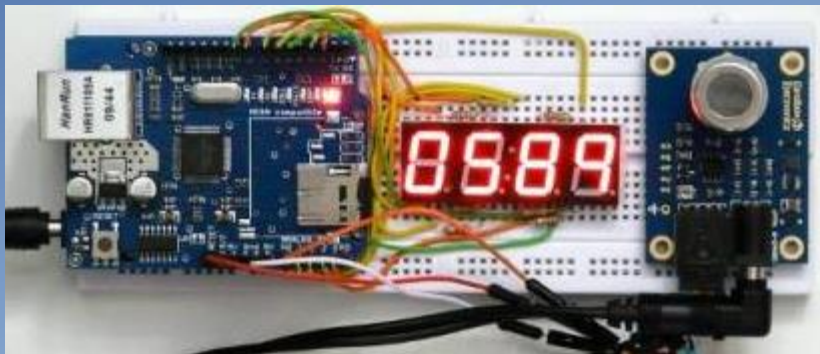
MG-811 CO 2 Gas Sensor Module and Arduino Microcontroller (2)
